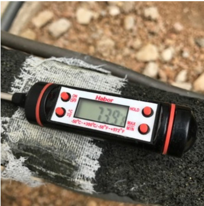
ELEVATED SUCTION LINE TEMP
