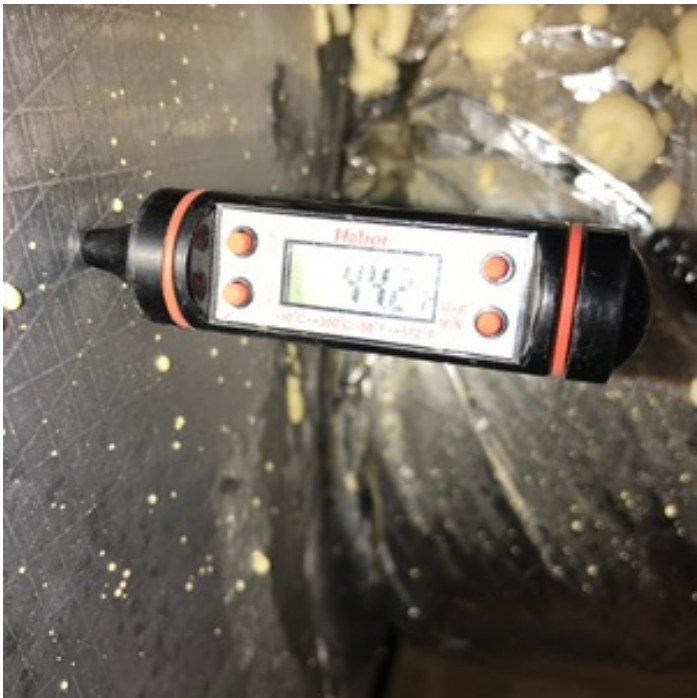
SUPPLY DELTA OUTSIDE RANGE (MARGINALLY)
