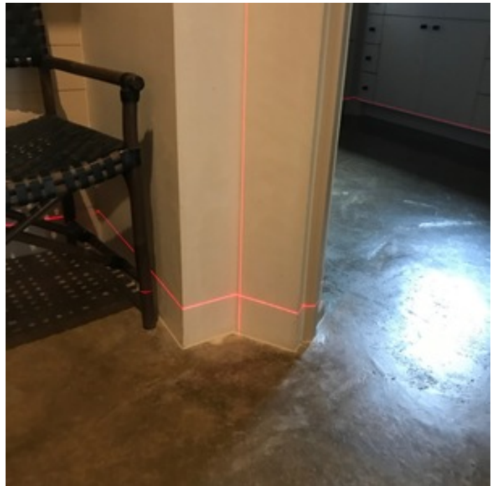
LASER LEVEL - TESTED WALLS PLUMB
