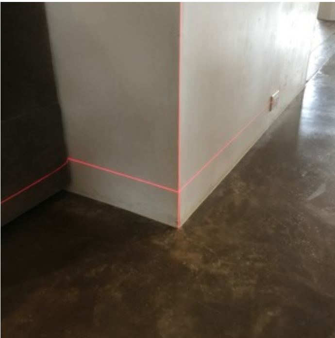
LASER LEVEL - TESTED WALLS PLUMB
