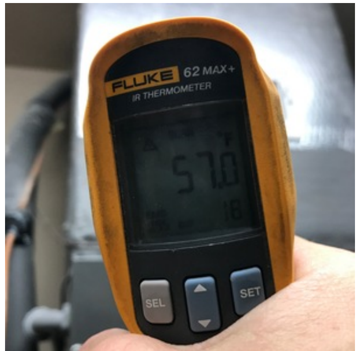
NORMAL SUPPLY TEMP - LOWER UNIT
