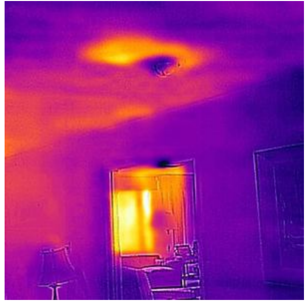
LOW INSULATION (OARNGE AT CEILING)
