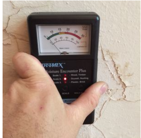
NORMAL LEVEL AT PREVIOUS LEAK
